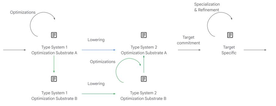
Frontend configuration: *order* of type system and substrate changes + target selection Default optimization pipelines can be informed by the target.
